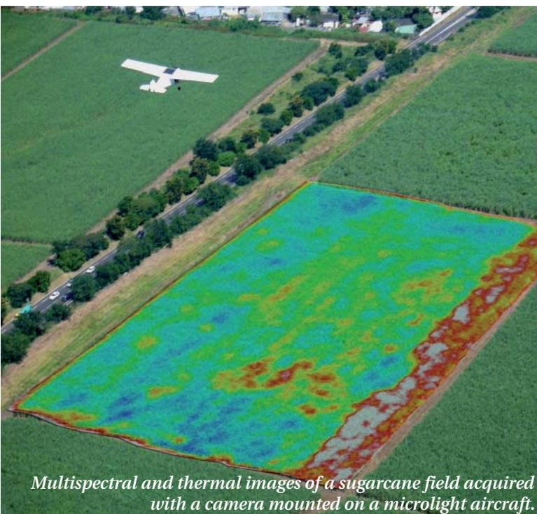
*Multispectral and thermal images of a sugarcane field acquired with a camera mounted on a microlight aircraft.*
