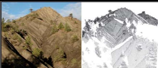
▲ Left: panoramic photograph; Right: 3D point cloud obtained by terrestrial lidar.
